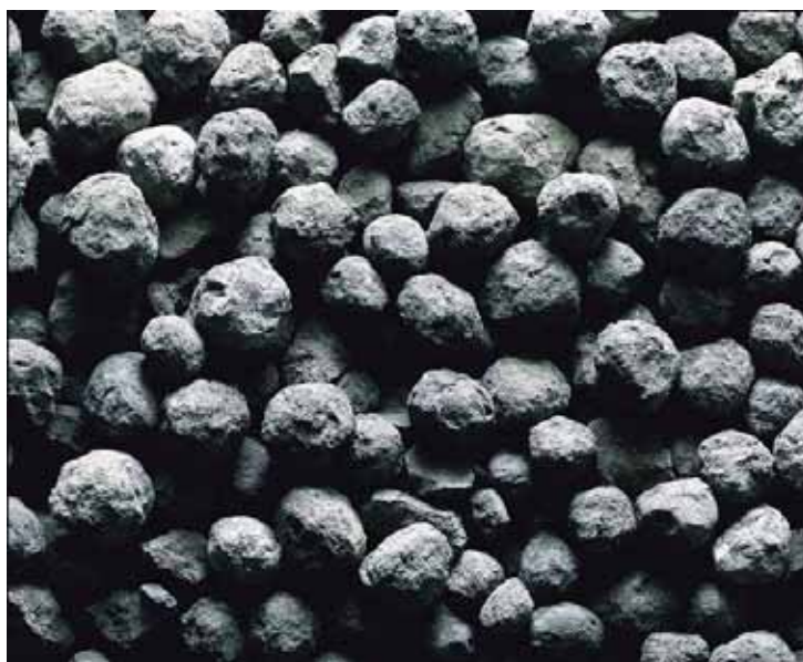
Figure 1-9: Photograph of cooled Clinker
