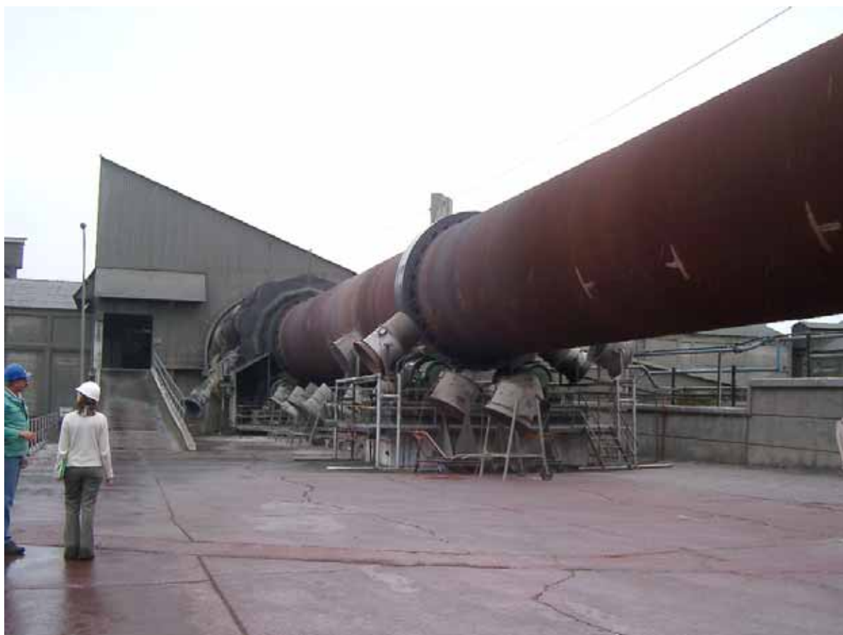
Figure 2-4: Photograph of the kiln at PE, showing the fans which cool the exterior of the kiln, and the control room housed in the background.
