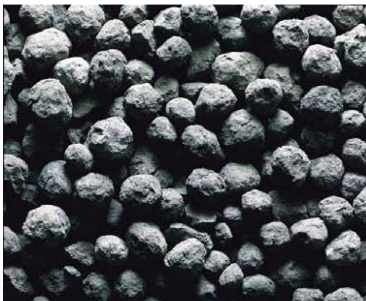
Figure 2-8: Photograph of cooled Clinker.
