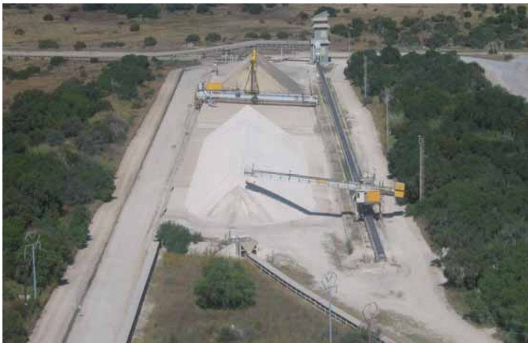
Figure 2-4: Photograph of the limestone stockpiles at Slurry. At the quarry, the limestone is crushed to particles approximately 25mm in size and stored on stockpiles, where the material is homogenised prior to milling.
